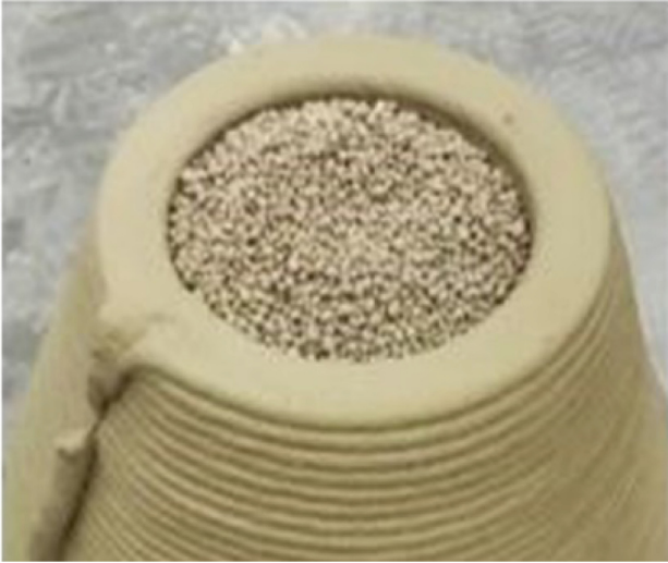
Fig. 7. Example of printing process without a confinement box.
