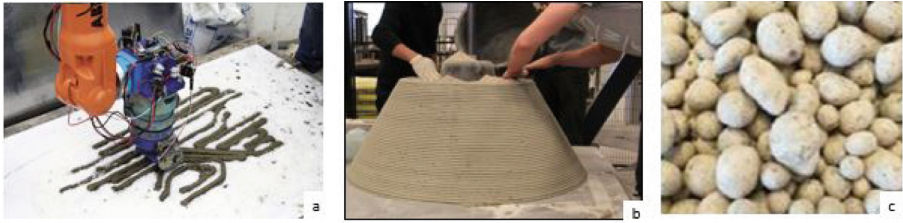
Fig. 5. Example of supporting material: (a) Concrete printing with salt as supporting material (Retsin and Garcia 2016). (b) Sand as supporting material (Salet et al. 2017). (c) Lightweight granular aggregate.
