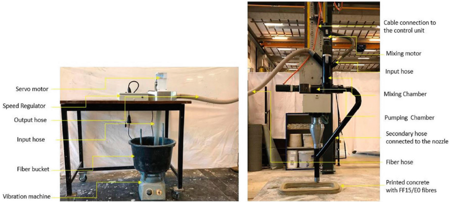
Fig. 8. Fibre reinforcement entrainment device (FRED) (Ahmed et al. 2020)
