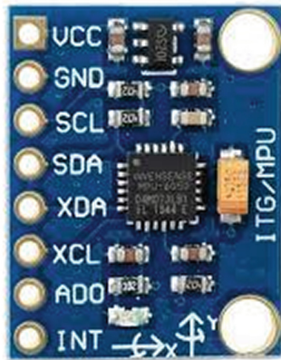
Fig. 8. 3-axes accelerometer and a 3-axes gyroscope
