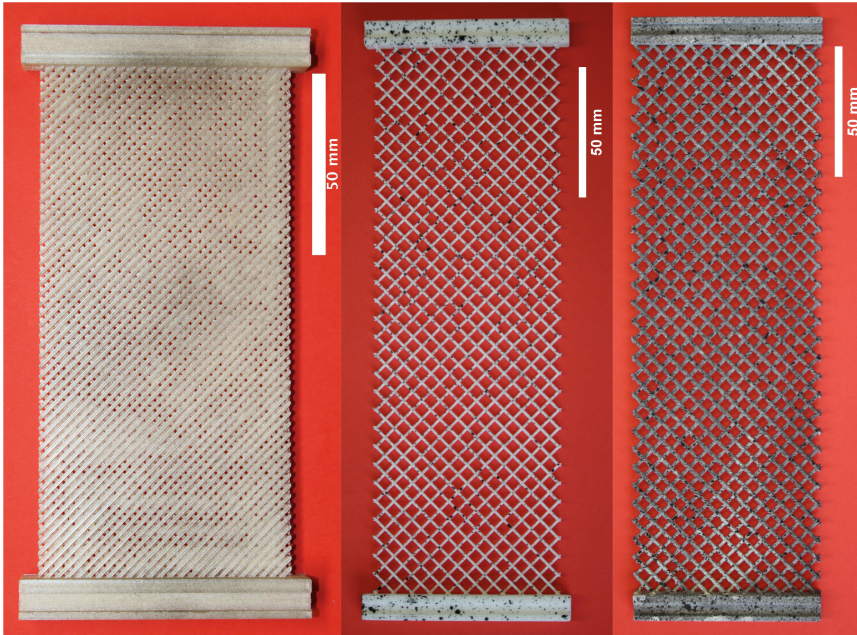
Fig. 3. Speckled pantographic structures made out of PLA (left), PA (middle), and AlSi10Mg (right).
