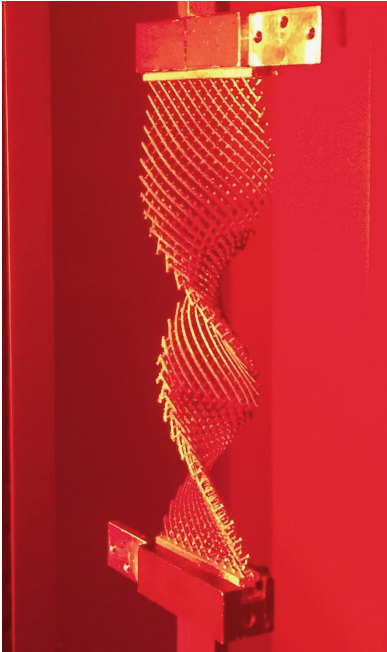
Fig. 10. Sample ALU-H after one full rotation during torsion test performed on Zwick Z010 at JWI, Charité in Berlin, Germany.
