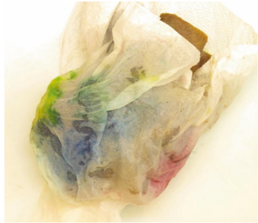
Fig. 3.6 Fixation of inks on the specimen surface: acetic acid is sprayed onto the inked surfaces through a thin paper towel to avoid running of colors due to the jet of the spray
