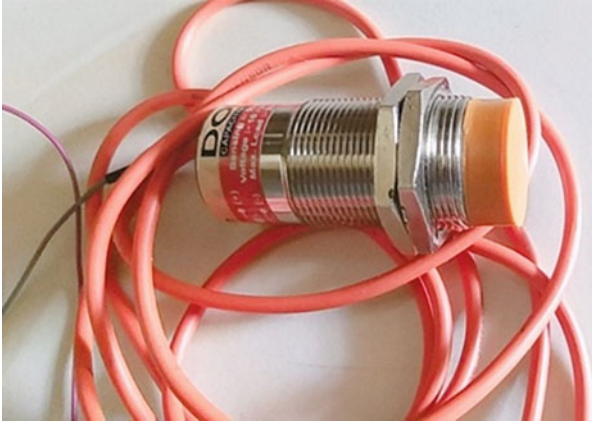
Fig. 13.12 Capacitive proximity sensor
