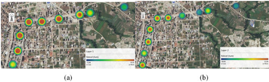
Fig. 70.3 Signal strength change with distance: dry case. (a) 1800 MHz (b) 900 MHz
