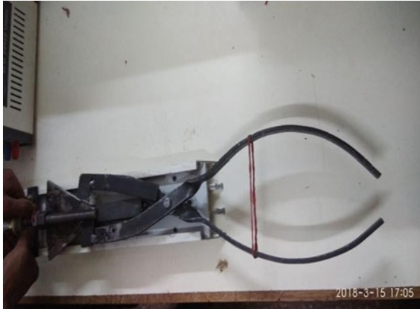
Fig. 37.2 Cam design for pineapple gripping
