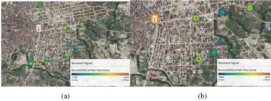
Fig. 70.4 Signal strength change with distance: rain Case. (a) 1800 MHz (b) 900 MHz
