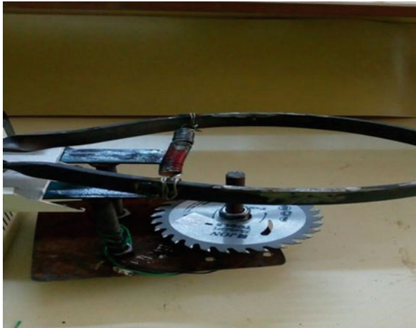
Fig. 37.3 Cutter design for a pineapple cutting
