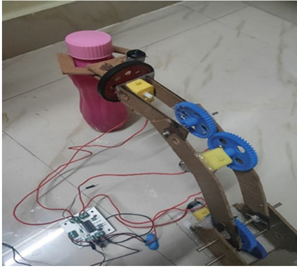
Fig. 13.15 Picking the object if it is plastic
