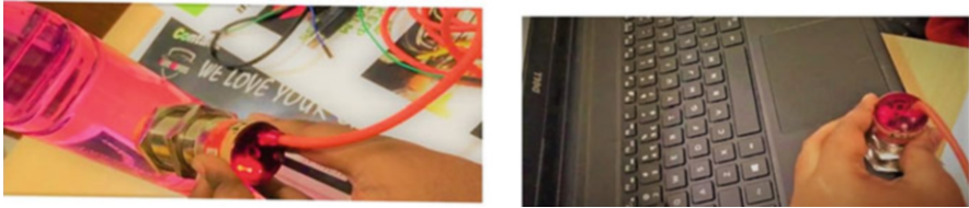
Fig. 13.13 Detecting the plastic by a capacitive proximity sensor
