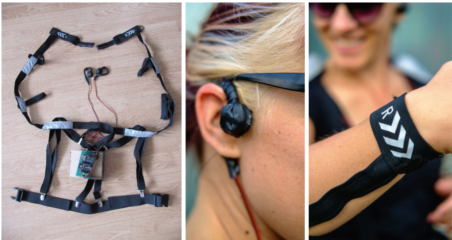
Fig. 3. Assembly of the final prototype (left), Open-ear headphone detail view (middle), wristband detail view (right).
