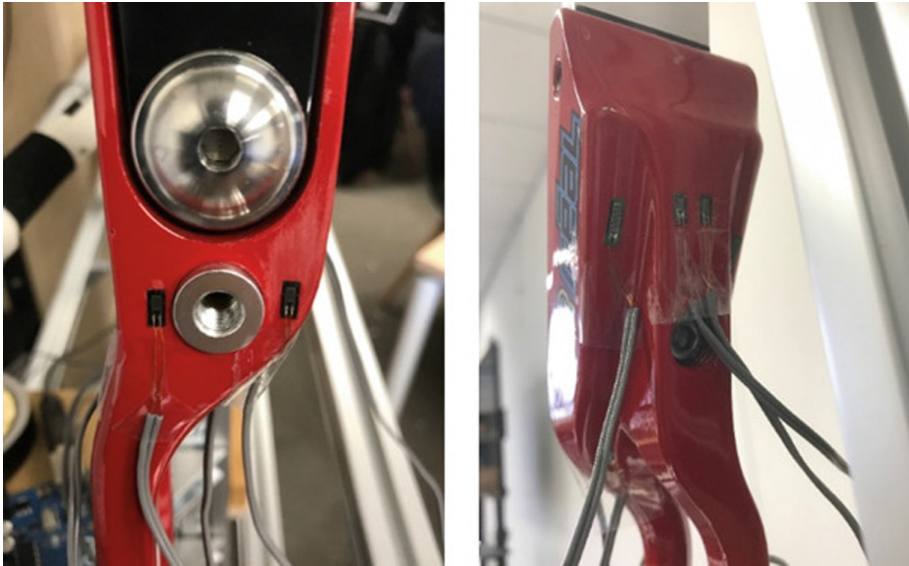
Fig. 9. Strain gauges attached over entire surface and back of upper and lower grips
