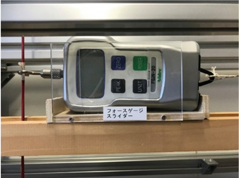
Fig. 7. Force gauge slider and ruler attached to measuring device, and string-pulling force can be measured
