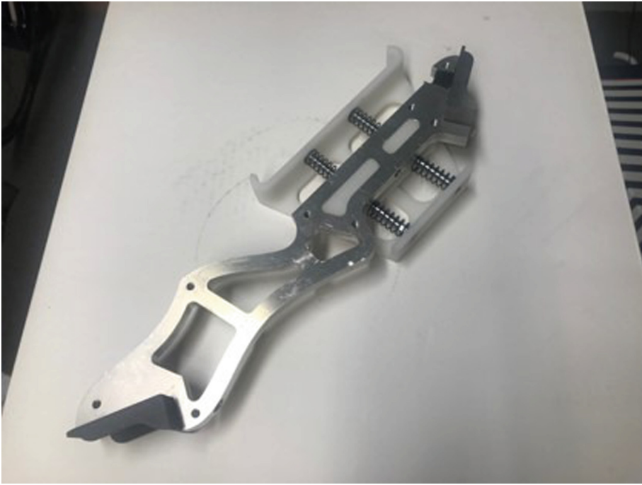
Fig. 15. Shock absorber consisting of shaft, linear bushing, and spring
