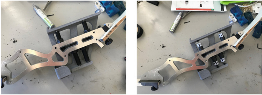
Fig. 14. Shock absorbers were fixed in 4 places between aluminum frame and base to fix vive tracker, and type of shock absorber was changed during experiment
