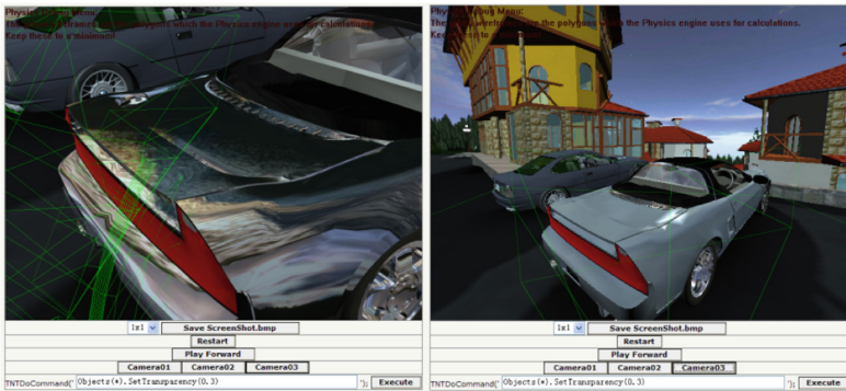
Fig. 2. Scene without and with a collide-able and permanently invisible box in online 3D GUI.
