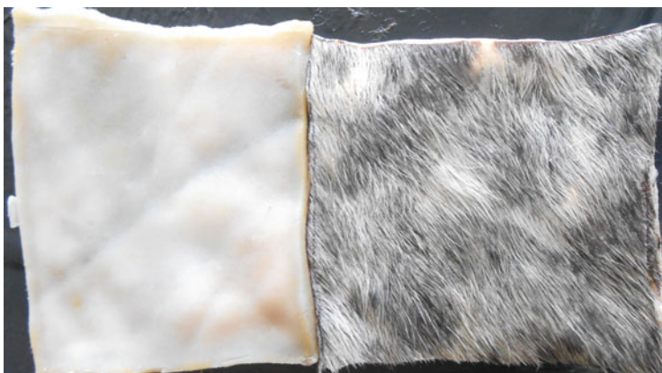
Fig. 3 Photograph of hide completely dehaired by crude alkaline protease within 3 h (pH 12 and 37°C); negative control where distilled water under the same condition remained with hair
