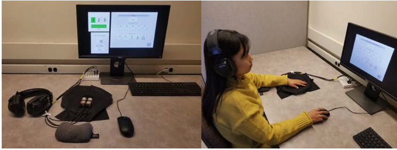
Fig. 7. Experimental setup: (left) noise-reduction headset, the palmScope display, elbow support, computer monitor, and mouse; (right) a participant in the middle of the affective rating experiment.
