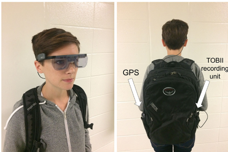
Fig. 3 Tobii Pro Glasses 2 mobile eye-tracking unit setup
