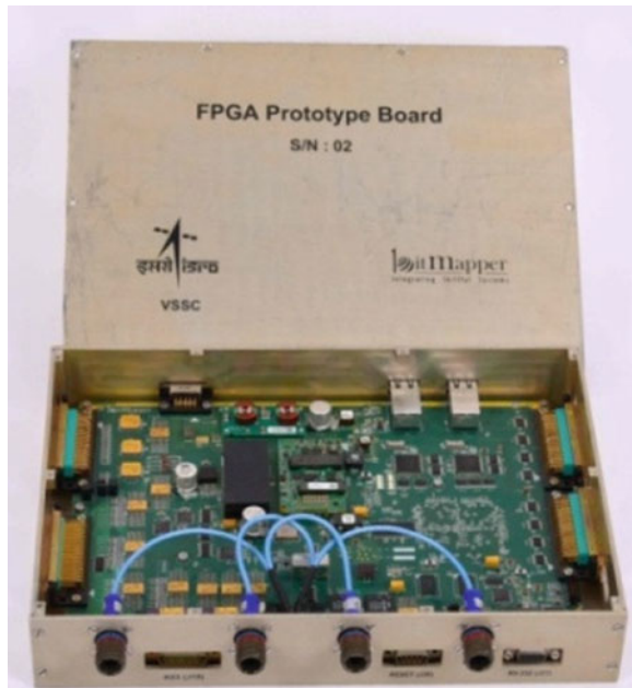
Fig. 4 FPGA prototyping board for tests
