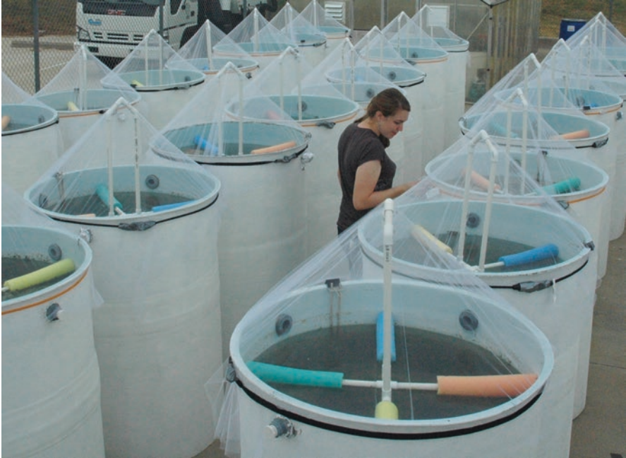
Fig. 4 Our experimental mesocosms are 550 l conical fiberglass tanks (0.6 m 2 surface area) located at the Texas Christian University mesocosm facility in Fort Worth, Texas, USA. Water is supplied from a nearby pond. The mesocosms were aerially colonized by aquatic insects and stocked with fish. Sediments collected from nearby ponds (LBJ National Grasslands, Decatur, TX, USA) contaminated with Hg from the atmosphere were added to the tanks to serve as a source of Hg. In Jones et al. (2013), mesocosms were covered with mesh netting to capture all emerging insects
