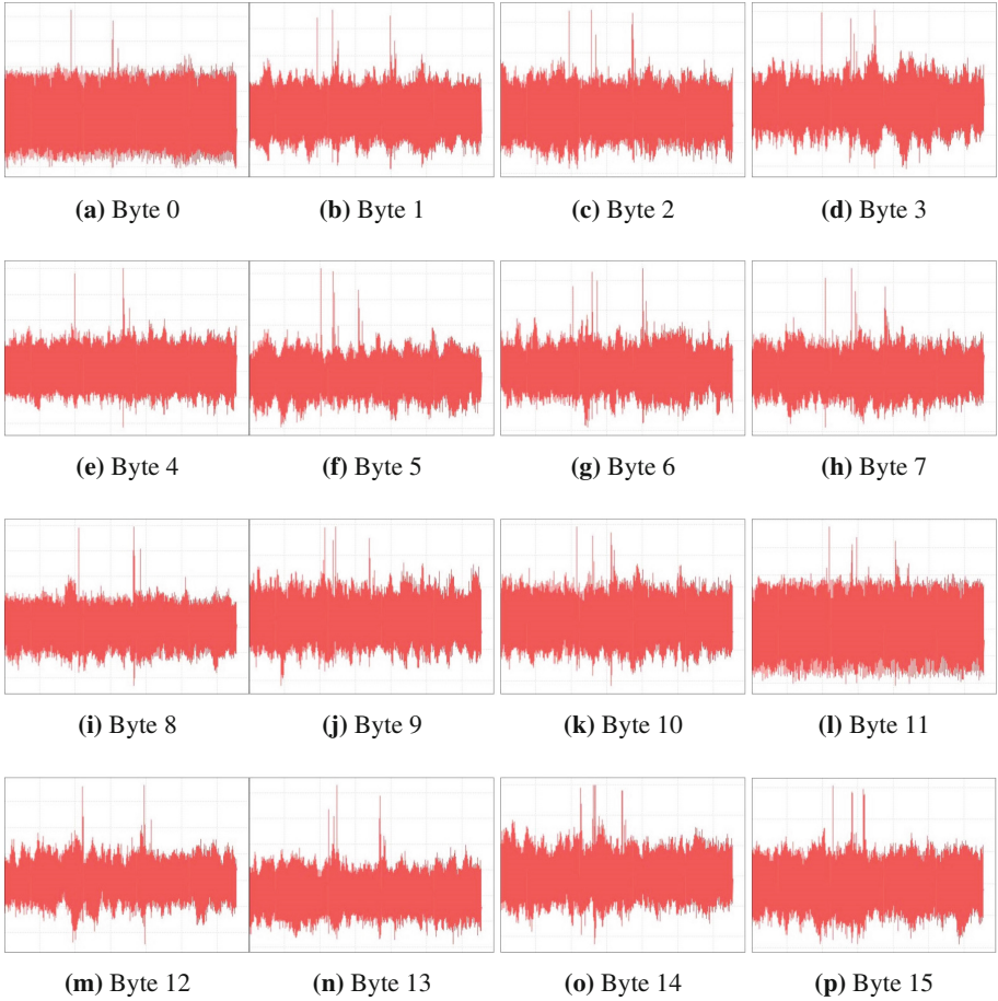
Fig. 5. Correlation between the EM-leakage and Hamming weight for each byte of recovered key k^* .
