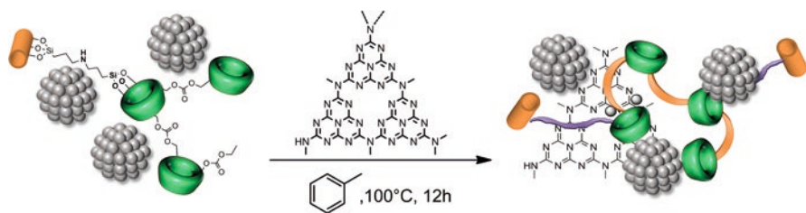
Fig. 5.28 The procedure for the preparation of Pd@Hal-CDNS- g -C 3 N 4 . As shown, cyclodextrin nanosponges (CDNS) was first prepared and amine functionalized and then reacted with Cl-functionalized halloysite nanoclay. In the next step, the as-prepared hybrid was palladated and hydrothermally reacted with g -C 3 N 4 . It is believed that cyclodextrin nanosponges served as a phase-transfer agent, while g -C 3 N 4 could suppress Pd leaching. (Adapted from Sadjadi et al. 2018b)
