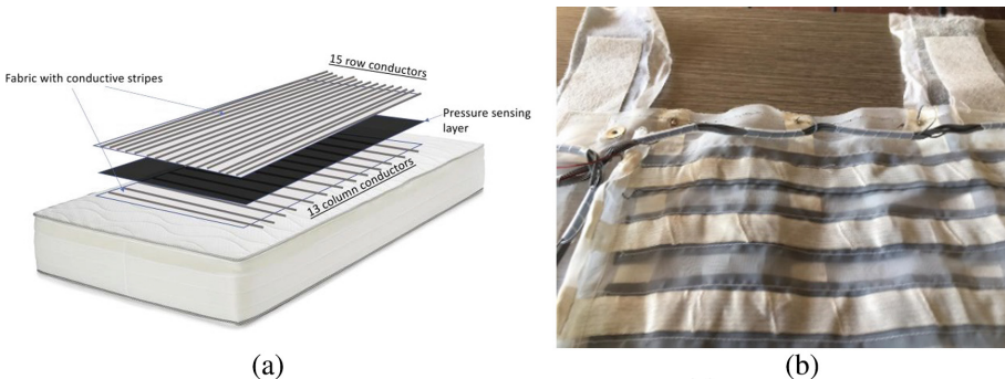
Fig. 1. a) Inner layer of CARBOTEX 03-82 (black layer, currently crawled in the direction of the lines); external PET layers with conductive stripes of row (15) and column (13) arranged orthogonally between them. b) Internal layer of CARBOTEX 03-82 cut into strips (black part); horizontal row and vertical column conductive tracks (silver parts) sewn onto the PET layer.
