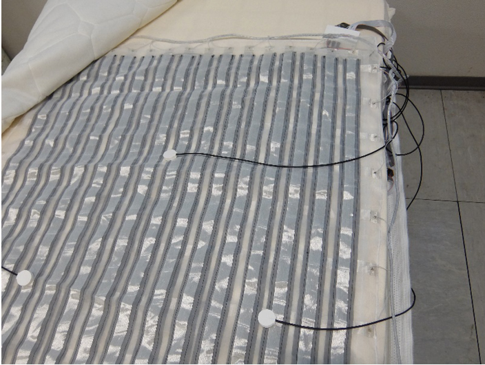
Fig. 2. Position of accelerometers (white dots) over the pressure matrix.
