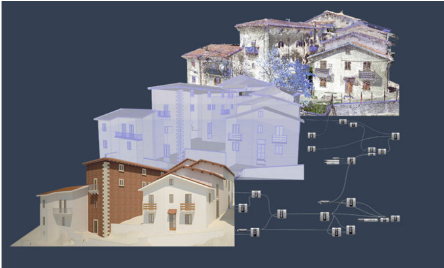
Fig. 8 BIM model of a Terracino’s urban aggregate realized through Visual Programming Language. The procedure is responsive and the model is updated and displayed in real time. Model by Adriana Caldarone
