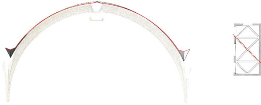
Fig. 11 Comparison between the diagonal section of the NURBS model (in red) and that deriving from the point cloud
