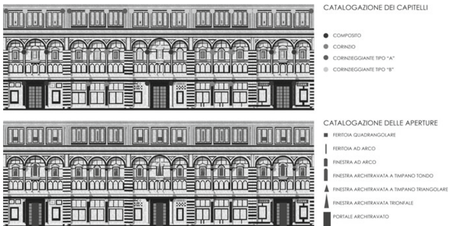
Fig. 3 Hierarchical identification of architectural elements. Elaboration by author on orthophoto
