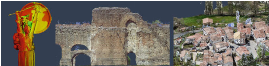
Fig. 1 Level of accuracy.’s macro categories. From left: high, medium and low. The level of accuracy, according to which the acquisition is conducted, does not depend on the size of the object, but on the level of detail that is desired based on the objectives
