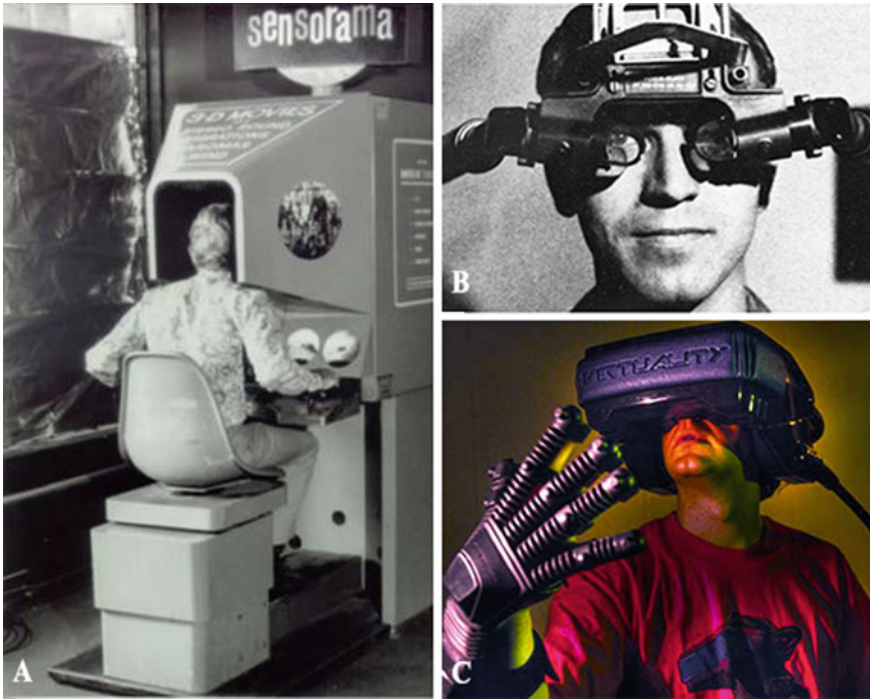
Fig. 2 A Sensorama, the first virtual reality machine; B Damocle's sword, the first virtual reality system with headset (so heavy it had to be supported by a structure); C Virtuality headset and glove. Credits A, B & C: Bianchini, Riccardo, "Quando i musei diventarono virtuali" in Inexhibit , 10/06/2016
