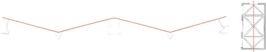
Fig. 13 Comparison between the longitudinal section of the NURBS model (in red) and that of the point cloud along the ridge rib
