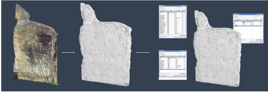
Fig. 2 Mesh information process of a claudio aqueduct’s barrel-vault. The aim of the client was to calculate geometric barycenter, enter information regarding materials and compute the volumes to be restored for securing. Level of geometry is more important than level of Information
