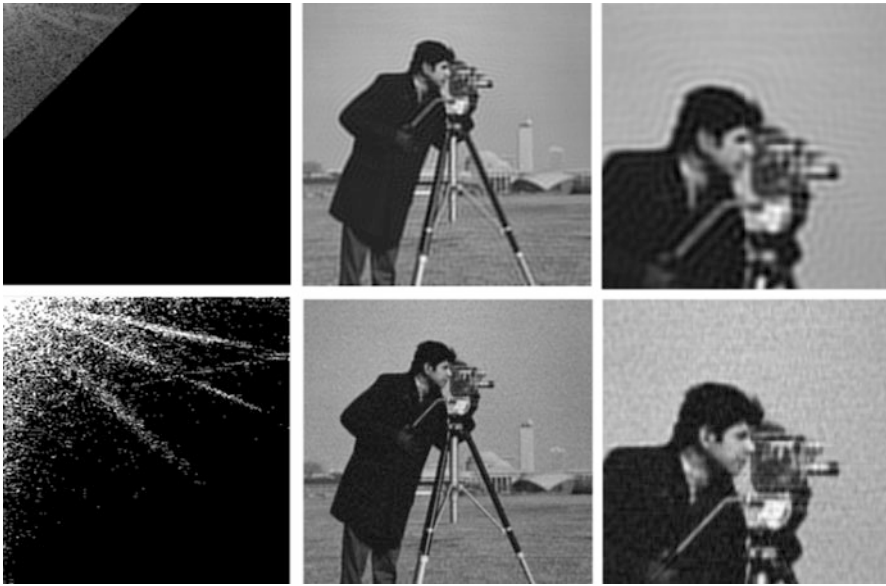
Fig. 16.14: Example of image filtering (compression) in domain of 2D DCT coefficients: (top) zonal filtering—only DCT coefficients from some matrix zone are left, (bottom) threshold filtering—only DCT coefficients exceeding some threshold are left [17]
