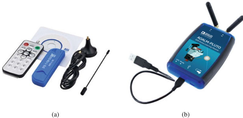
Fig. 17.6: Two very cheap software defined radio hardware platforms. (a) RTL-SDR USB stick (FM/DAB/DVB-T) [10]. (b) Analog Devices PLUTO active learning module—figure from [11]
