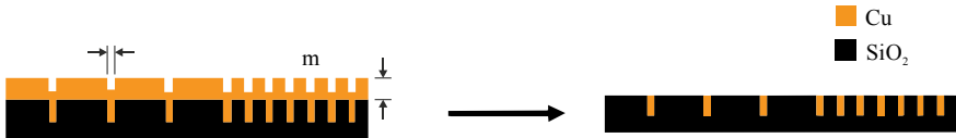
Fig. 6.2 Etched wafer after copper deposition (left) and after removing the copper layer by the CMP process (right). Reproduced with permission from Melvin (2003b)
