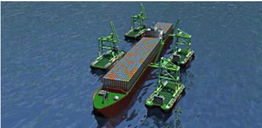
Fig. 1.5 Mobile harbor concept invented at KAIST (four mobile harbors are unloading containers from a large ocean-going containership in open sea to transport the containers from the ship to the shore)
