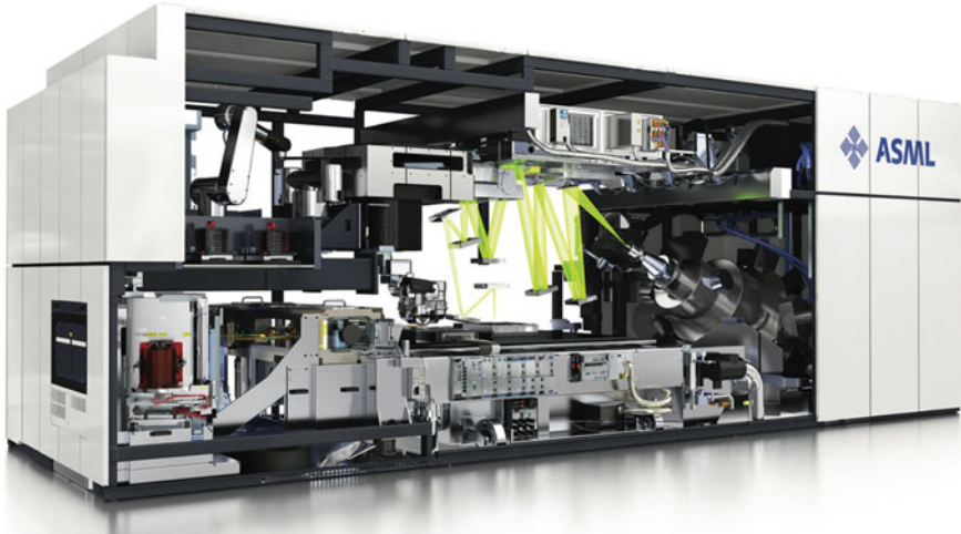
Fig. 3.12 A lithography machine for semiconductor wafer manufacturing (Permission granted by ASML)
