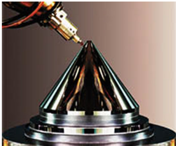
Fig. 8.2 Surface generated by the Large Optics Diamond Turning Machine (LODTM). (Courtesy of Lawrence Livermore National Laboratory (Klingmann 2001))
