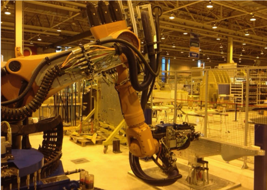
Fig. 18.6 Drilling and fastening robots
