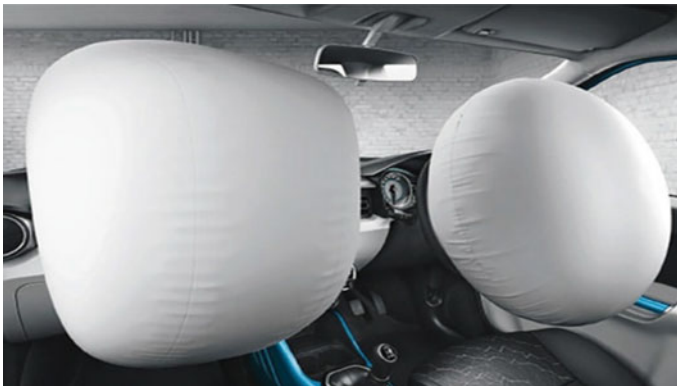
Fig. 6.5 Airbags of nylon 6.6
