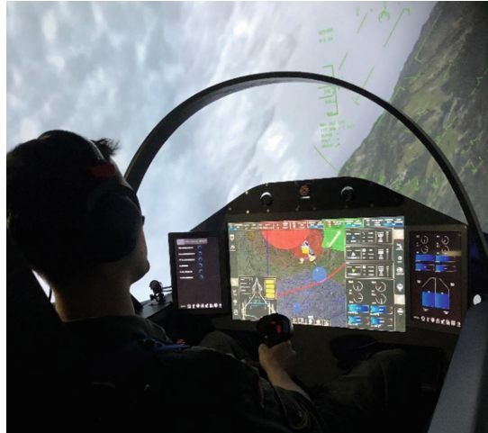
Fig. 2. Generic fighter jet cockpit simulator of the Institute of Flight System.
