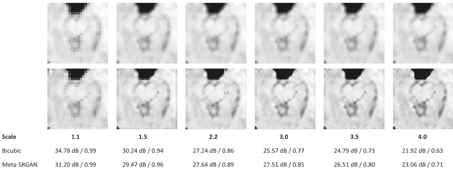
Fig. 8. (Top) Image going through various upsampling factors using Bicubic Interpolation. (Bottom) Image going through various upsampling factors using Meta-SRGAN. PSNR and SSIM scores are calculated against a target image downsampled by a factor of 4.
