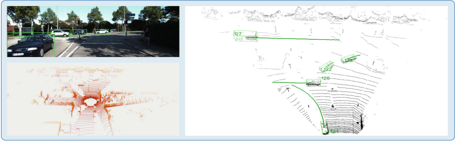
Fig. 1. Proposed 3D detection and tracking coupling system result. Left top image and left bottom image shows the 2D detection results and the raw points cloud as input. Right image shows the 3D detection and multi-object tracking result. Objects' trajectories are represented as deep green curve, green numbers are IDs of each object. (Color figure online)
