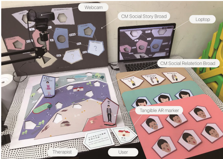
Fig. 2. The physical setup of the ARCM social-training system
