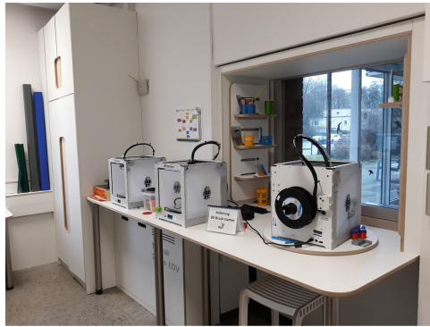
Fig. 2. 3D-printer work area with one rotating plate and glass panel
