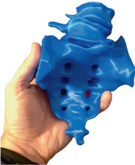
Fig. 8.7 1:1 scale FDM 3D printed sacrum derived from CT data (print material PLA, print time 34 h)
