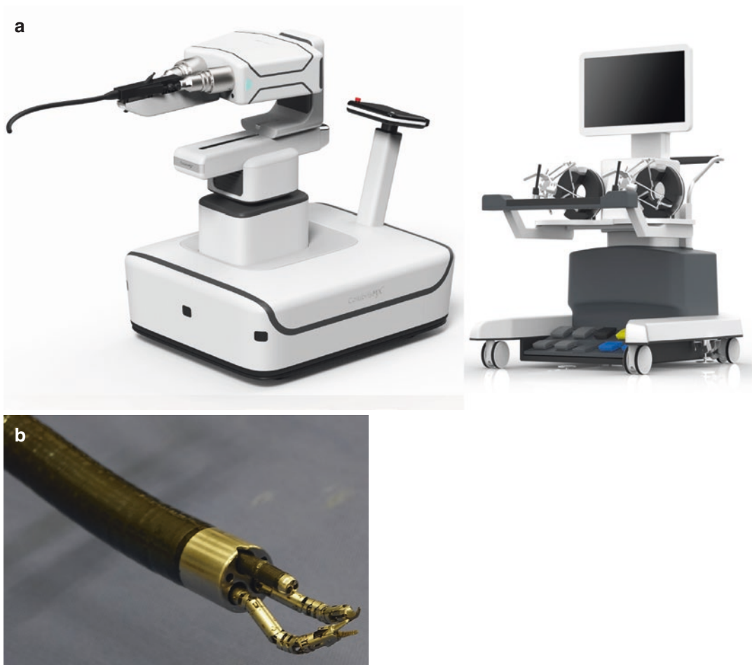
Fig. 22.14 An emerging surgical system, the endoluminal surgery (ELS) system, by ColubrisMX Inc. (Houston, TX) is an advanced, robotic endoluminal system currently undergoing clinical validation. (a) The console worksta-
