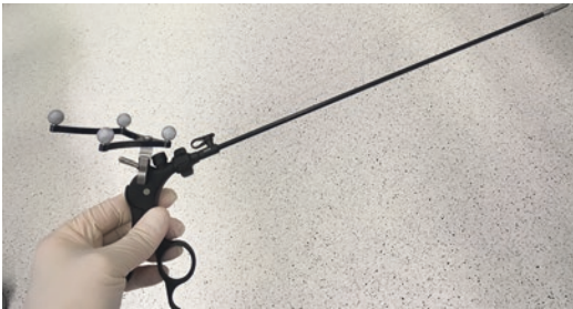
Fig. 11.3 The tip of a surgical instrument can be tracked by means of an instrument tracker which is fixed to the instrument. It can be attached to an energy device or a regular surgical instrument. (From Romagnolo et al. [28]. Reprinted with permission from Springer Nature)
