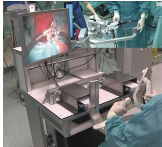
Fig. 22.13 The Single-Access Transluminal Robotic Assistant for Surgeons (STRAS) robot is shown. This master-slave, robotically assisted system enables tele-operated endoscope handling by a single surgeon and allows for colonic submucosal dissection. The endoscope is inserted manually and connected to the slave system (inset). It houses three working channels for instruments, of which one can accommodate standard endoscopic tools. After insertion, the two tele-operated instruments are controlled by the surgeon seated at a workstation, as shown. (Photo courtesy of IRCAD France, iCube Laboratory Strasbourg, and KARL STORZ, reproduced with permission)
