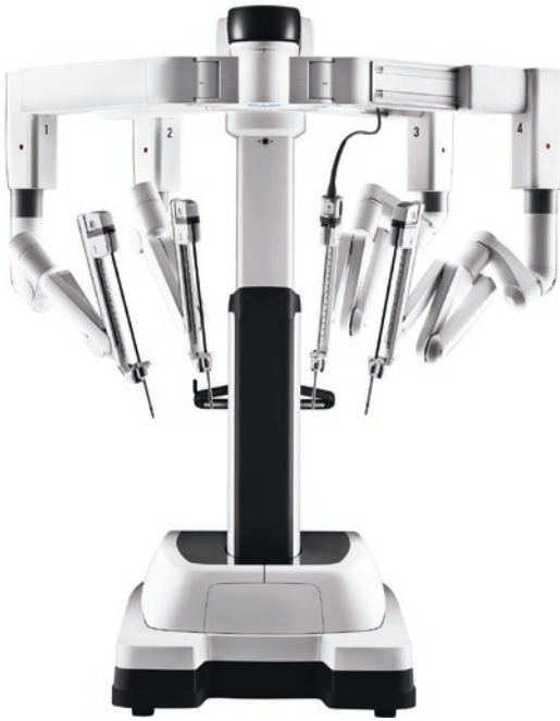
Fig. 32.4 Da Vinci Xi. It has four arms that are beneficial for multi-quadrant procedures [40]. (©2020 Intuitive Surgical, Inc. Used with permission)
