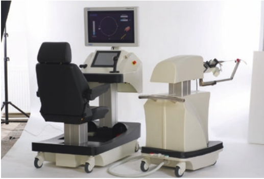
Fig. 22.12 Avicenna Roboflex (ELMED™ Medical Systems Company, Orlando, FL, USA) is a flexible robotic ureteroscope. The master-slave device allows precise scope control and can perform all tasks performed with conventional ureteroscopy. It is operated by a urologist seated at a workstation (shown) that includes dual joysticks with scope drive controls. Proponents of the devices believe it is useful for lithotripsy, enhancing stone fragmentation and dusting. It may also reduce operator fatigue due to improved ergonomics, and at the same time, physician exposure to ionizing radiation is minimized. (Photo provided with permission and courtesy of ELMED™ Medical Systems Company)
