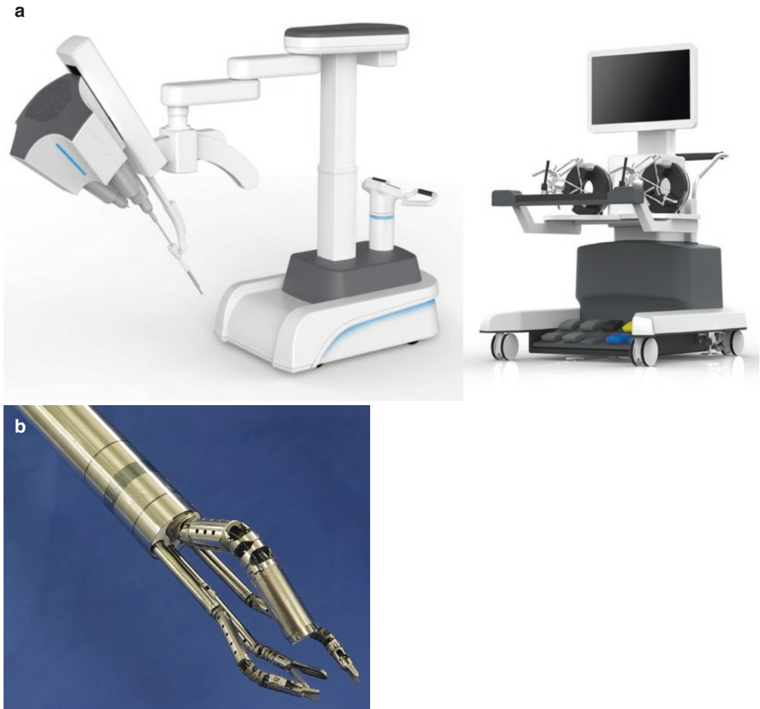
Fig. 30.1 (a) An emerging robotic single-port system by ColubrisMx with open console and single boom robotic beside cart is shown. (b) Close-up detail illustrating the
