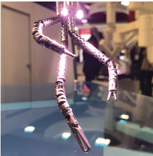
Fig. 22.2 The da Vinci SP Surgical Robotic System is shown. The system deploys three working arms (6 mm dia. each) as well as a stereoscopic 0° camera head via a 2.5 cm cannula. The camera and instrument effector arms have both elbow and wrist flexibility; the system is prototypical for nonlinear robotics in surgery. Such a framework is suited for access to difficult anatomic targets that demand systems which can follow a curved pathway
