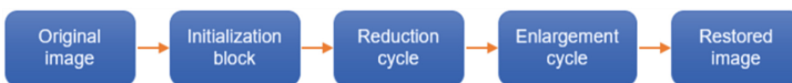
Fig. 1. Block diagram representative of the Gaussian Pyramid method to restored range image.
