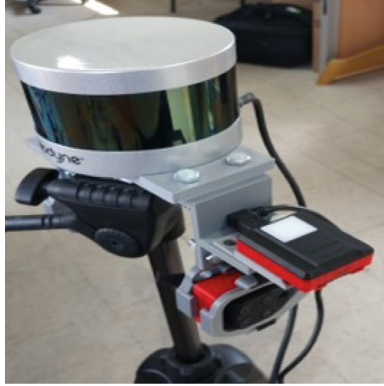
Fig. 3. Our LiDAR-camera rig, consisting of a VLP-16 LiDAR and a Sequoia Multi-spectral camera. (Color figure online)
