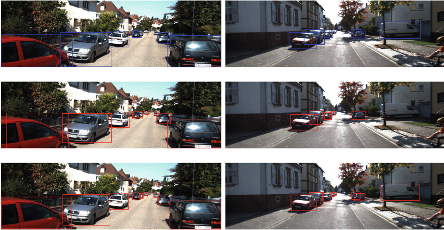
Fig. 2. Groundtruth (first row), YOLOv3 detection (second row), Detectron2 detection (third row) are presented. It is possible to observe that Detectron2 adjusts bounding boxes better and detects cars that Yolov3 does not.
