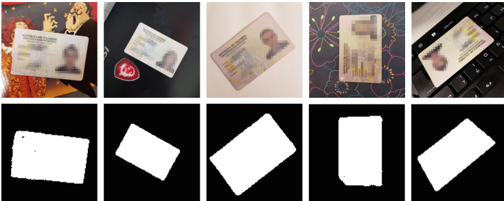
Fig. 4. Document localization process by using image semantic segmentation. Upper images are original pictures and lower images are the deep learning generated masks.
