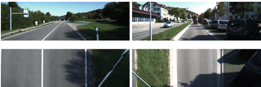
Fig. 4. BEV transformation results. The original image (first row) and Bird's Eye View transformation (second row) are presented.
