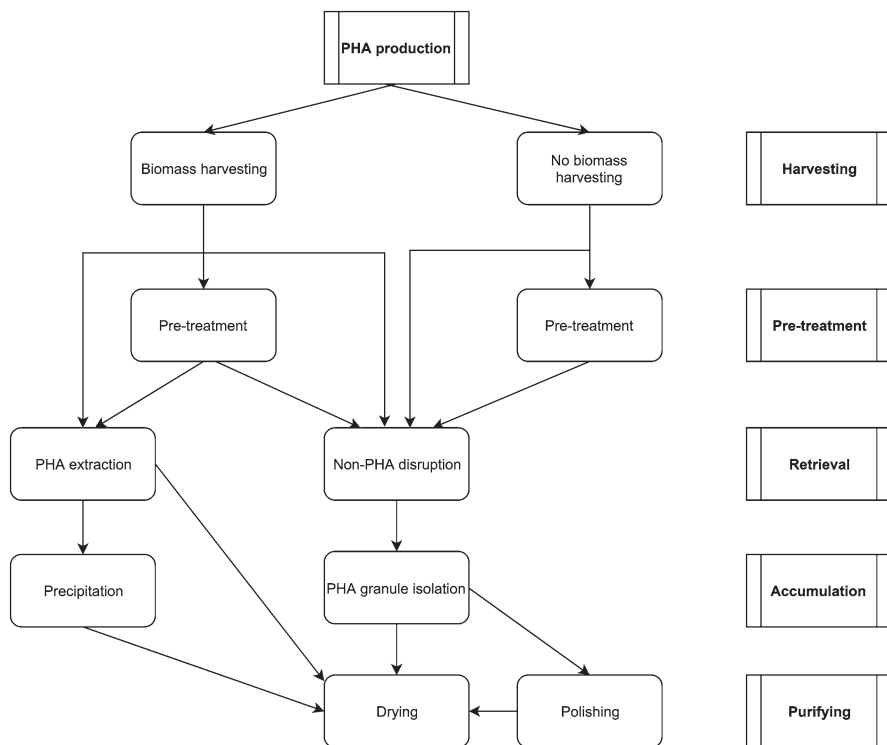
Fig. 5.6 Polyhydroxyalkanoates recovery system
