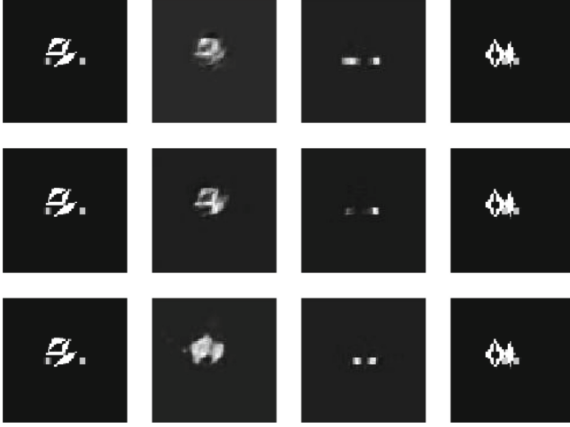
Fig. 9. Example of the influence of kernel size and stride. First column: pre-close image, second column: object channel prediction, third column: gripper channel prediction, fourth column: post-close, ground truth image. First row: result of model 1 (kernel sizes I, filters I, stride 1), second row: result of model 2 (kernel sizes IV, filters I, stride 1), third row: result of model 3 (kernel sizes I, filters I, stride 2).
