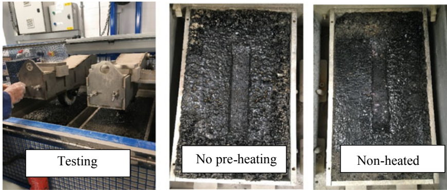
Fig. 4 Modified Hamburg wheel tracking test
