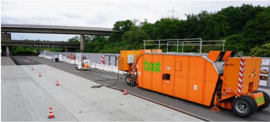
Fig. 6 Mobile Load SimulatorMLS30 on duraBAST
