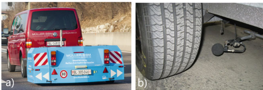
Fig. 2 CPX system measuring in flowing traffic (a) and view on microphone installation (b)
