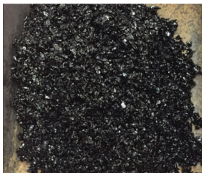
Typical Pothole Patching Mix
