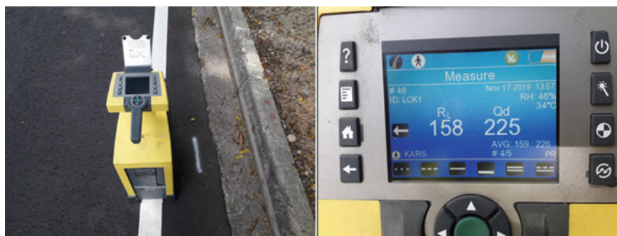
Fig. 6 Retroreflectometer result shown real-time
