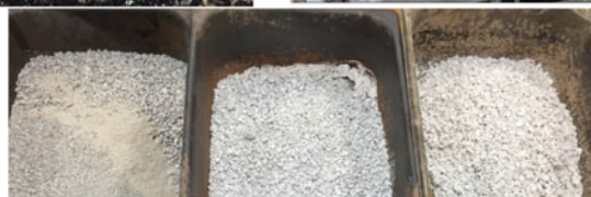
Aggregate Residue from Typical Patching Materials
