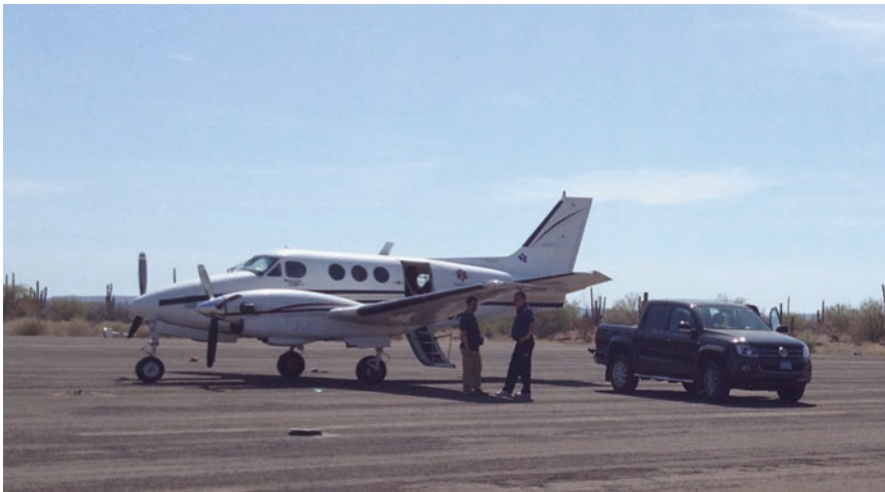
Fig. 2 This Beechcraft King Air C-90 turboprop fixed wing pressurized aircraft awaits a patient near Mulegé, Mexico. This type of aircraft has range up to 1000 miles (1609 km) and cruises at 245 mph (394 kph). (Photo Credit: Jay Doucet, 2012)
