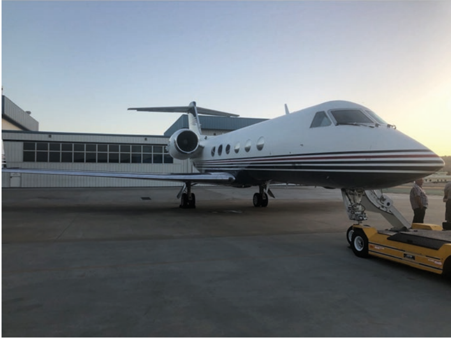
Fig. 3 This Gulfstream IV air ambulance is a pressurized jet with a range of over 4800 miles (8000 km) and cruises at 552 mph (888 kph). It can perform transoceanic air evacuations. (Photo Credit; Jay Doucet, 2019)
