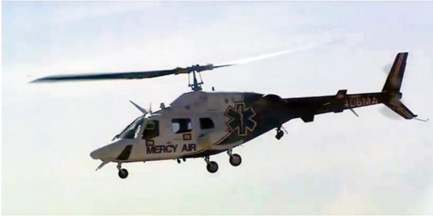
Fig. 1 This Bell 222B helicopter has a range of 434 miles (700 km) and cruises at 155 mph (250 kmh). It is unpressurized and typically carries a single patient, a flight nurse, and/or paramedic and a single pilot. (Photo Credit: Pat Choothesa 2012, with permission)
