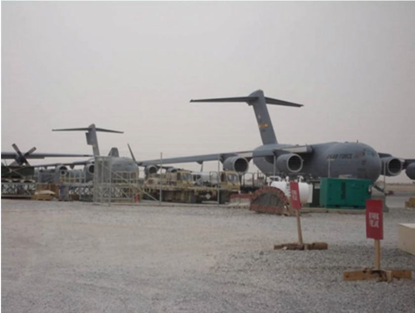
Fig. 4 US Air Force C-17 Globemaster III Transport aircraft stand by on the flight line at Kandahar Airfield, Afghanistan, to take Critical Care Air Transport Teams (CCAT) and their patients to Landstuhl, Germany. The C-17 has a range of 6456 mi (10,390 km) and cruises at 516 mph (830 kph). It can carry up to 36 litter and 54 ambulatory patients. (Photo Credit: Jay Doucet, 2006)
