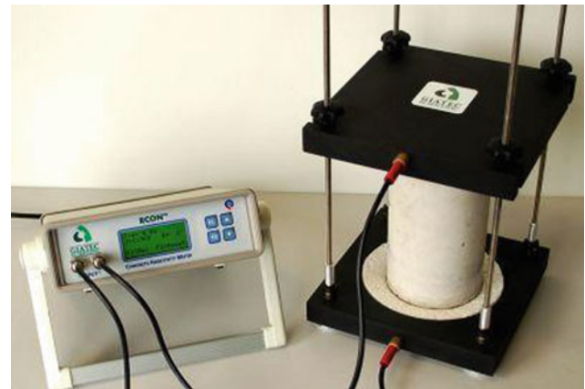
Fig. 4 Bulk resistivity measurement device
