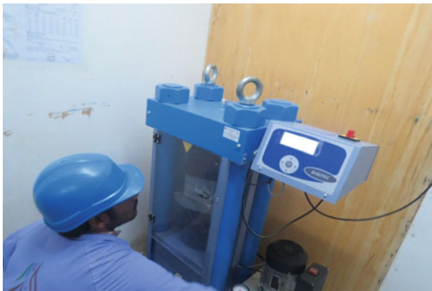
Fig. 4 Compaction Test of Different Cube Trough Compaction Testing Machine 219 (BS 1881-116:1983)
