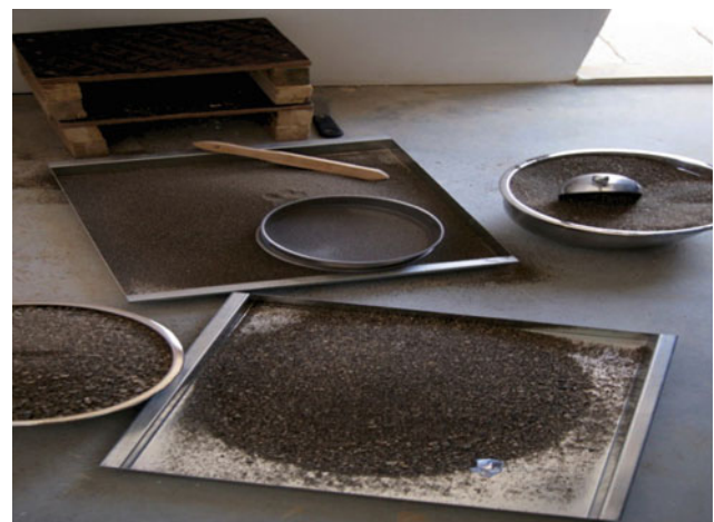
Fig. 2 Sieve Analysis for Fine and Coarse Aggregates (ASTM C136)
