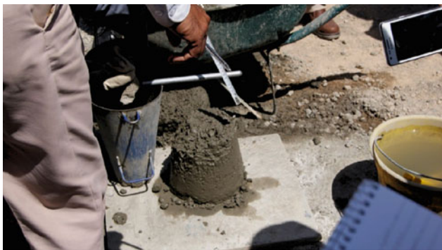
Fig. 3 Slump Test for Checking Workability (ASTM C143)
