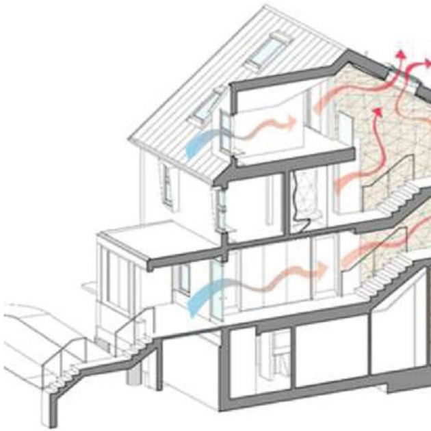
Fig. 5 Natural Ventilation System for a building including windows and skylights (Wu et al. 2018)
