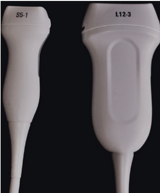
Fig. 1.3 Left, broadband sector array transducer with a frequency range of 5 – 1 MHz for trans-/intracranial insonation. Right, broadband linear array transducer with a frequency range of 12 – 3 MHz for transcutaneous/extracranial insonation
