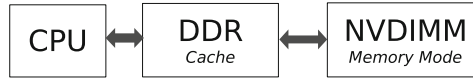
Fig. 2. 2-Level-Memory mode (2LM) uses DDR as a Memory-side Cache in front of the Memory Mode part of NVDIMMs exposed as normal volatile memory.
