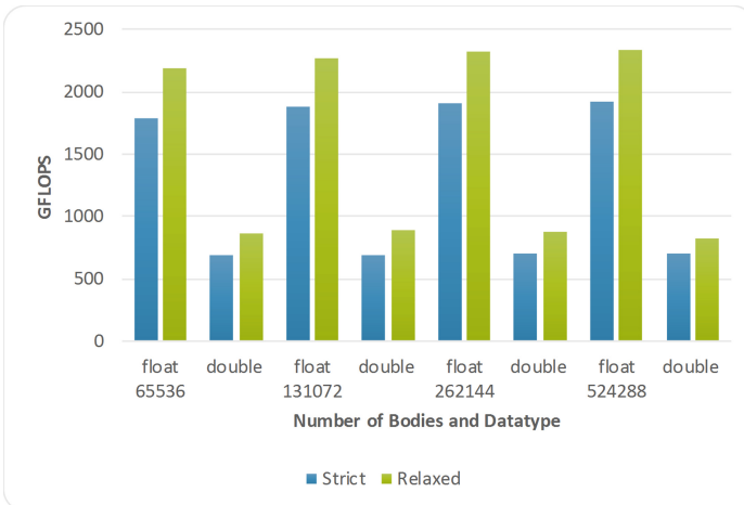
Fig. 6. Performance for precision relaxation when both the datatype and the number of bodies varies on the Xeon Phi 7230.
