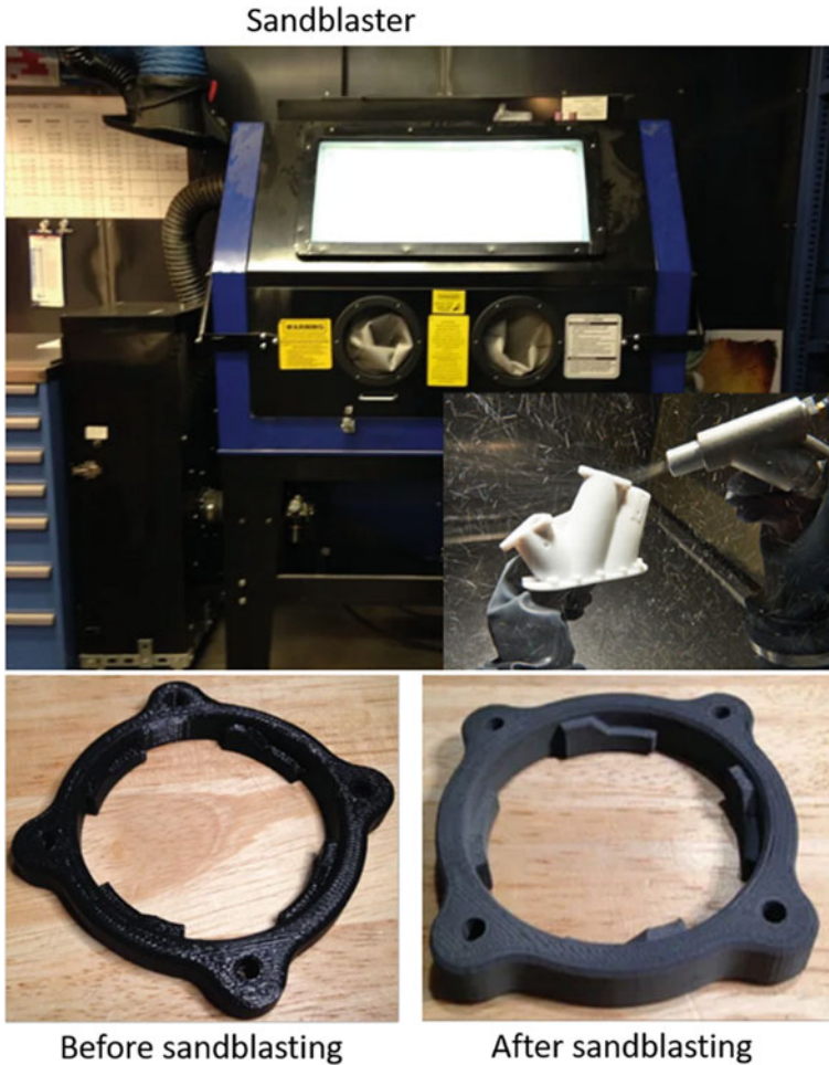
Fig. 4.4 Sandblasting of FDM parts. The surface quality transformation after sandblasting is also shown (obtained from open-access webpage: www.instructables.com ). The inset illustrates the process of the sandblasting inside the blasting chamber
