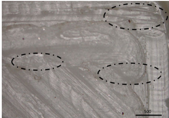
Fig. 4.2 a) The CAD design for the features and b) illustrating the incomplete melting and fusion at the beginning of the printing process (adapted from Mwema et al. [1])
