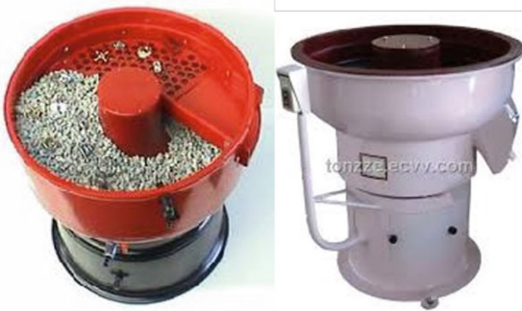
Fig. 4.7 Examples of grinding vibratory machines used in the finishing of FDM parts. Obtained from Stratasys Ltd. webpage ( www.stratasys.com )
