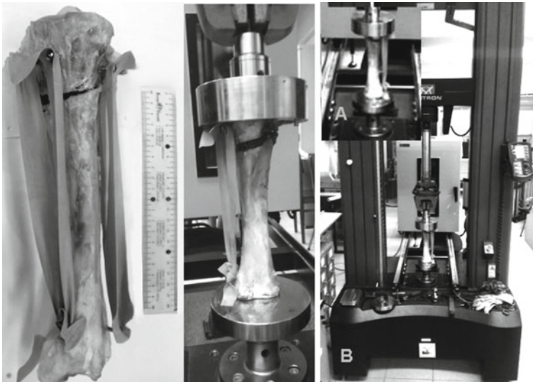
Fig. 4.8 High tibial osteotomy model (left) is installed to loading machines INSTRON 8801 (middle) and INSTRON 5982 (right)
