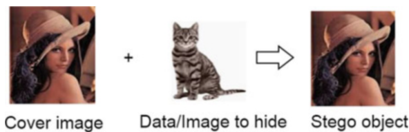
Fig. 17.1 General schemata of a steganographic procedure: a cover image will act as a carrier for the data to conceal. The data to hide, in this case, the cat figure, will set its pixel information on the cover image by modifying the bit information of their pixels. Another steganographic procedure could perform image transformations on the cover image. In either case, the result is a stego-object that contains the concealed data, which is not visible by simple inspection
