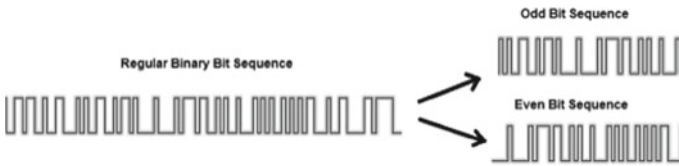
Fig. 6 Bit sequence broken to even and odd groups [13]
