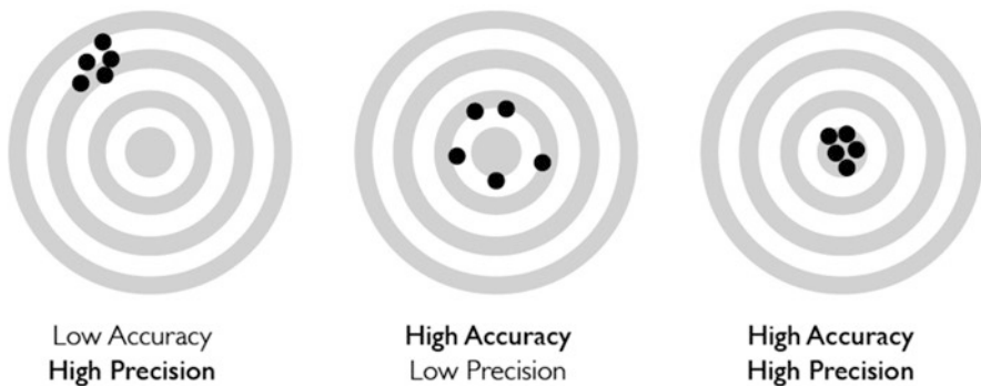
Fig. 6.4 An illustration of the difference between precision and accuracy
