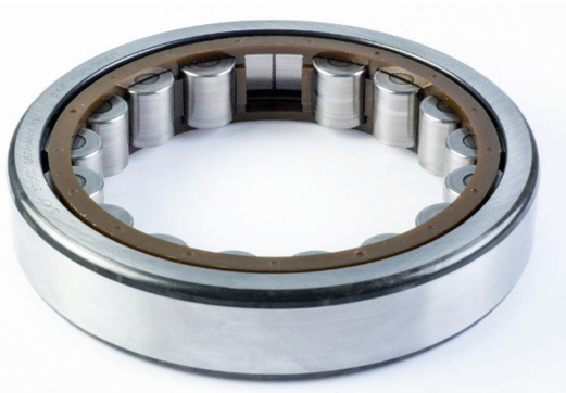
Fig. 1. NU220 ECP bearing used in testing, artificial damage seen in the outer race
