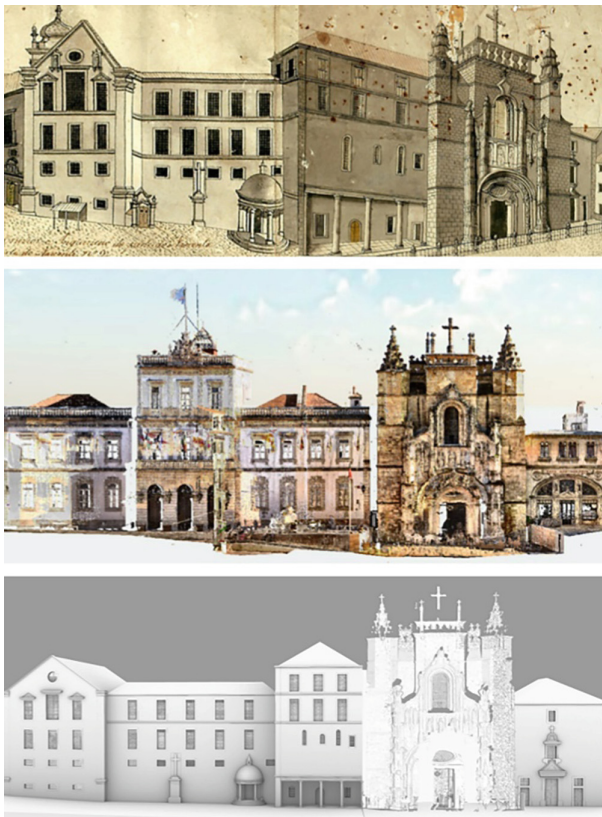
Fig. 1. Façade of Santa Cruz Monastery, drawing by José Carlos Magne (detail), 1796. Source: Machado de Castro National Museum, Coimbra. // Laser scan of current facades of the Coimbra town hall building and Santa Cruz church. Source: Santa Cruz research project. // Tridimensional model of the previous façade of the Santa Cruz Monastery (before 1834). Source: Santa Cruz research project (3D reconstitution by Antonio Monteiro).
