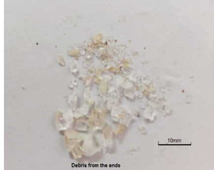
Fig. 5. Fracture of 8 mm specimen
