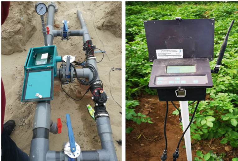
Fig. 1 Equipment of smart irrigation system titled “Intelligent Control System of Water Saving Irrigation”
