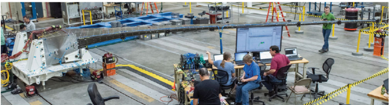
Fig. 7.8 The simplified modal test setup: the Passive Aeroelastic Tailored Wing mounted on only the Wing Loads Test Fixture reaction table
