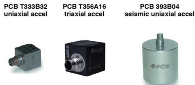
Fig. 7.10 Ground test accelerometers used for modal testing (not to scale)
