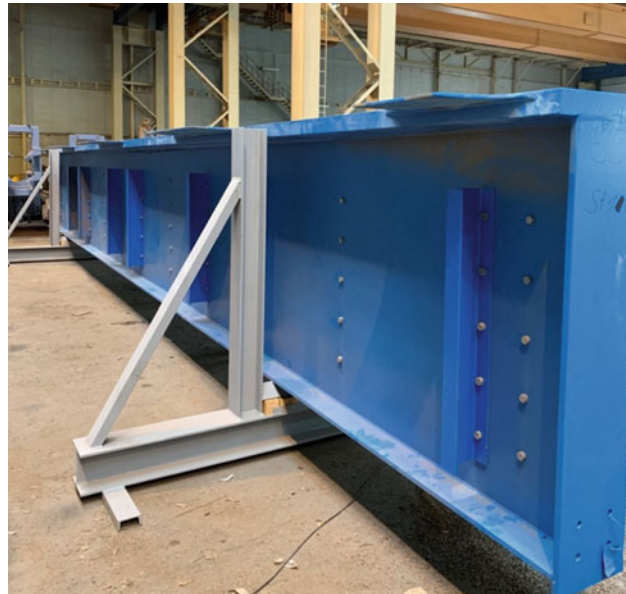
Fig. 37.5 Runway beam with downshop conductor fittings screwed on its both sides
