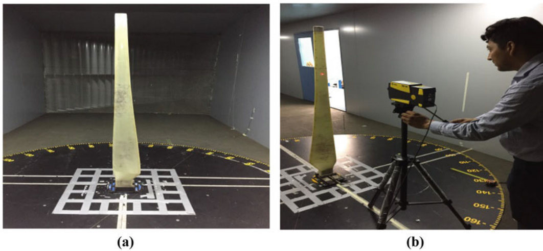
Fig. 1.2 Wind tunnel set up for modal testing of the wind turbine blade: (a) Free clamped boundary conditions and (b) Power-distance mount and focus stabilization of the portable laser vibrometer
