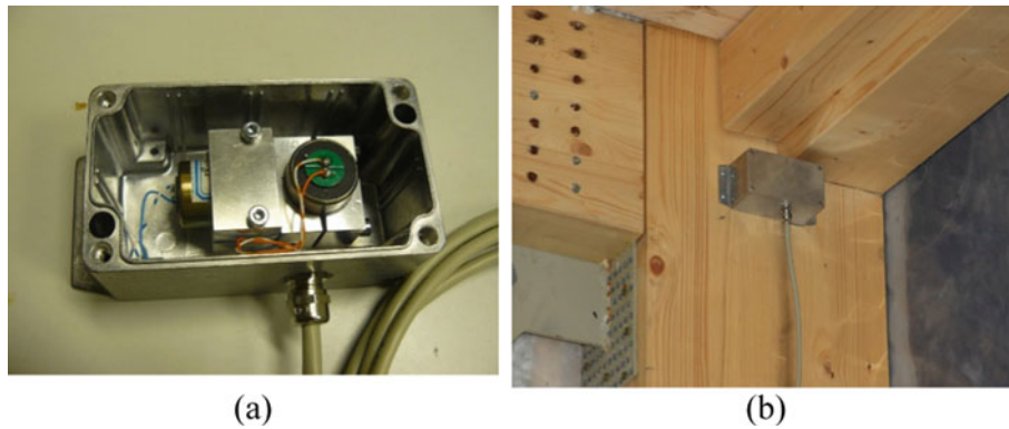
Fig. 14.3 Installation of geophones. (a) Two geophones inside a box. (b) The box attached to the structure
