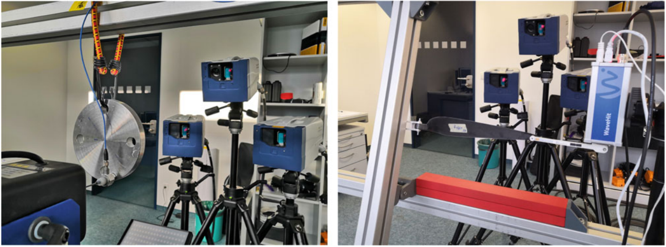
Fig. 9.4 Left: Setup for the Experimental Modal Analysis on a flange. The structure with free boundary conditions is excited by a shaker between 4–12 kHz. Acquisition of the system response via 3D-LSV. Right: Setup for the Experimental Modal Analysis on a rotor blade. The structure fixed on one side was excited broadly by an automatic modal hammer (WaveHit, gfaitech GmbH). Acquisition of the system response via 3D-LSV
