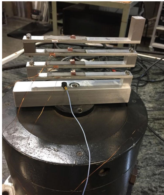
Fig. 21.4 Foldable harvester on top of vibration exciter table
