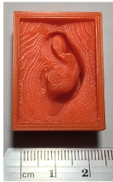
Fig. 6. Example of a 1:2 size left auricle mold (2 cm × 3 cm) as obtained using reverse engineering and a Zortrax M200 3D printer.
