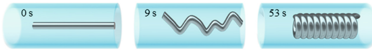
Fig. 2. The shape-memory-induced embolism overtime at 37 °C [20]. The blood vessel is represented as a cyan tube; the coil is in gray at 0 s, 9 s, and 53 s.
