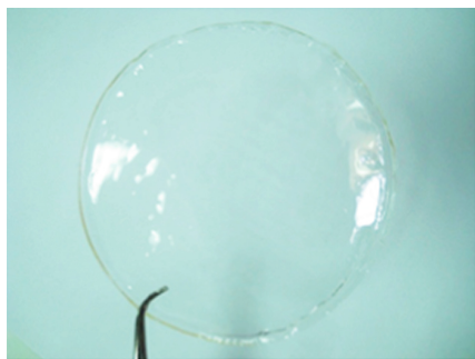
Fig. 1. PVC/PS60 based film realized by the solvent casting technique
