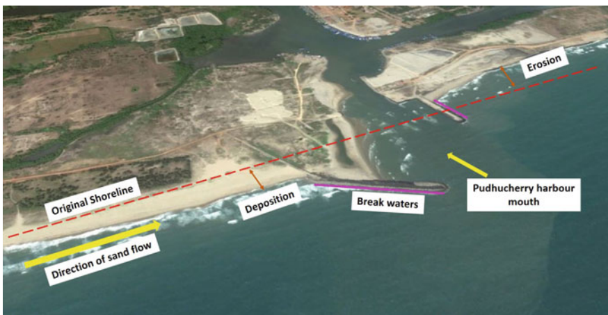
Fig. 6.1 Effect of hard coastal structures on a shoreline
