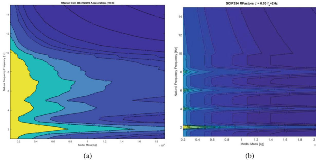
**Fig. 11.3** Contour maps of response factors in terms of floor modal masses and natural frequencies. Both maps were obtained with a constant damping ratio  $\zeta = 0.03$ . (a) R-Factor based on OS-RMS90 Accelerations. (b) Acceleration R-Factor following SCIP354
