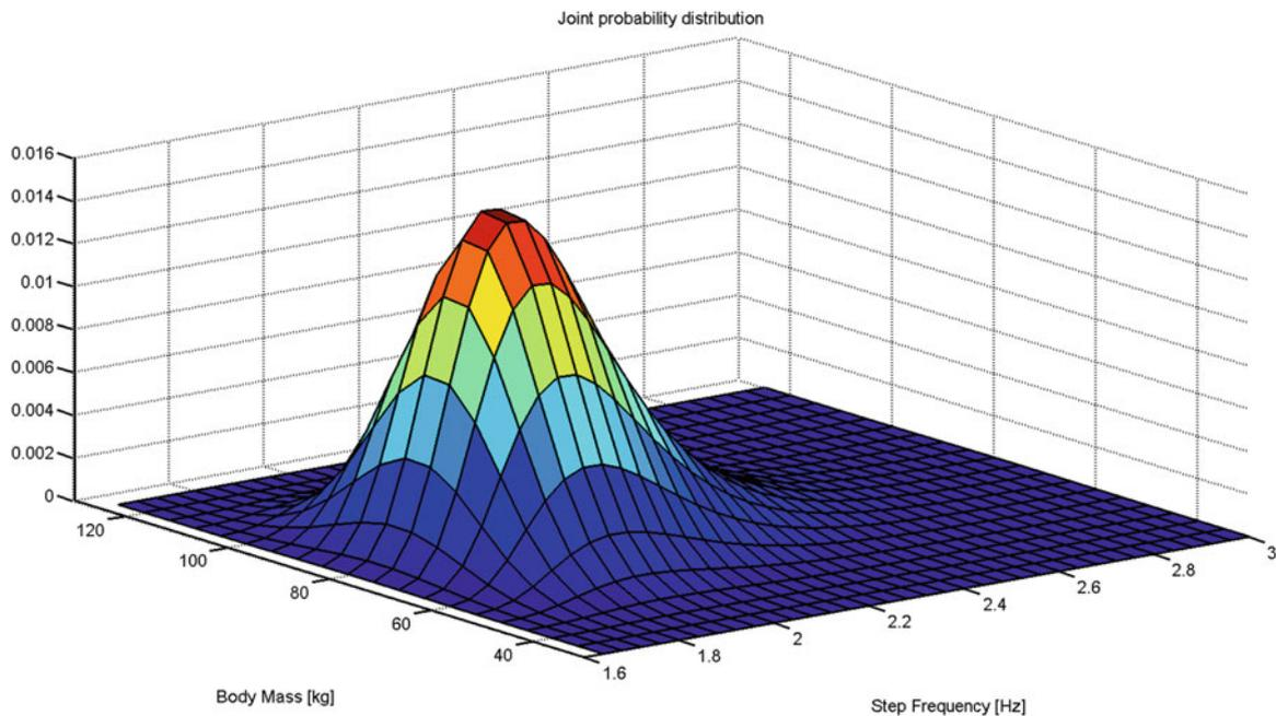
**Fig. 11.1** Body mass and step frequency joint probability distribution used as a statistical input for the OS-RMS method. This gives an expected frequency of 2.0 Hz and a body mass of 78.2 kg
