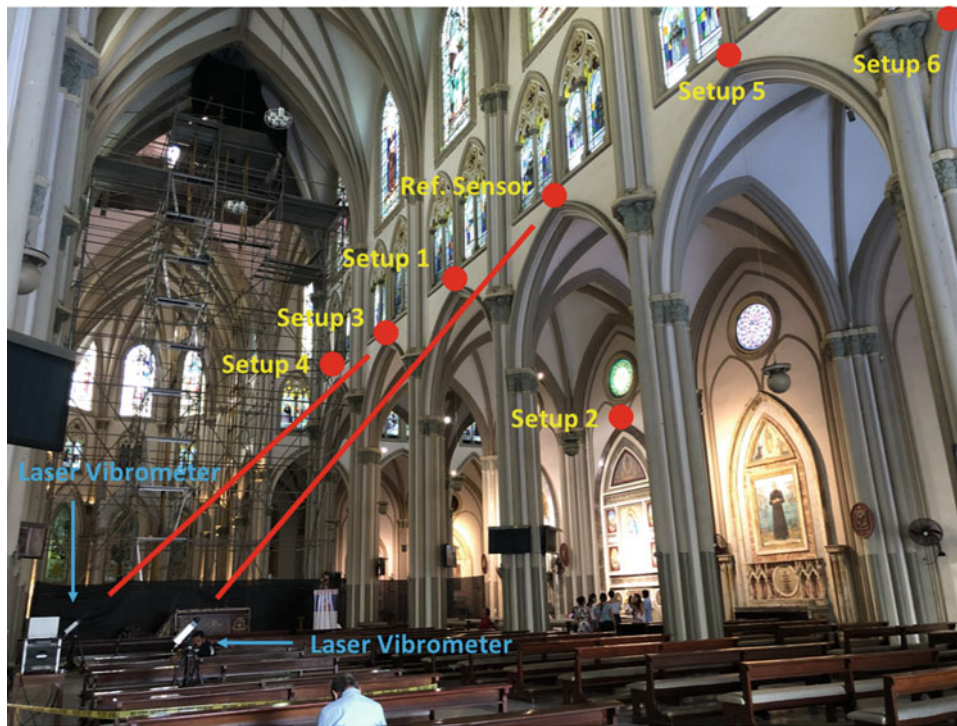
Fig. 9.2 Location of the Laser Vibrometers' target in Test 3 at the North Diaphragm (Setups 1–6)
